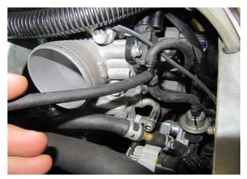
Vacuum Tee installs between the intake manifold behind the throttle body and the fuel pressure regulator. The long line goes to the blow off valve
